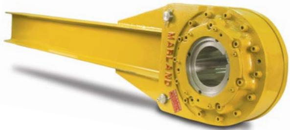
**Backstops BC-MA prevent reverse rotation on conveyor systems.** Marland has the broadest range of backstops in the marketplace with the newest designs having torque capacities surpassing the 2850 kNm mark (2,100,000 lb. ft.) and bore ranges to 600mm (23.6 in.). To meet the requirements of virtually any backstopping application Marland offers over 17 different models and a full range of shaft retention options.
